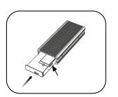
6. Install the PCB back into the track inside the housing. Pay attention to the correct alignment of the LED window!
