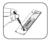
4. Then push the SSD card down and fix it with the delivered screw at the PCB.
